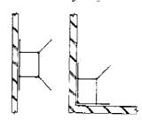
Where outriggers or Jumbo outriggers are fitted, as detailed overleaf, they must be used in one of the following ways if the tower has to be positioned against a wall or in a corner.
