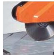
**INTEGRATED TRAY CHANNELS DIRECT WATER BACK TO THE PAN AND ALLOW QUICK POSITIONING OF THE MATERIAL AT A 45° ANGLE**
