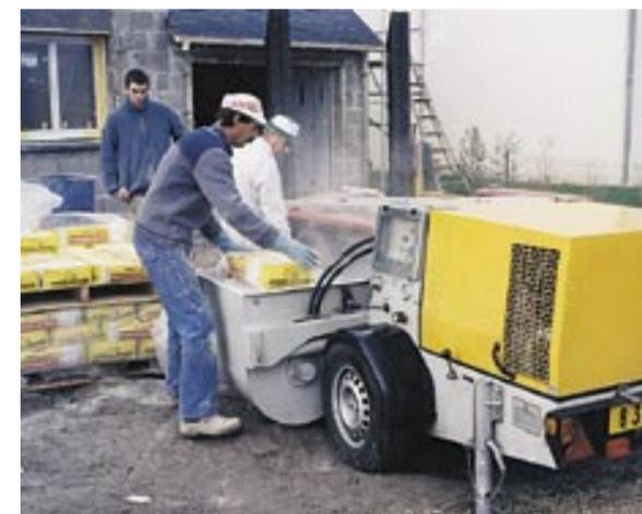
But that is by no means all! This SP 11<sup>DMR</sup> has a lift mixer with powerful hydraulics to carry out the job.
