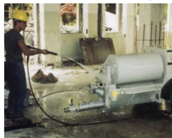
Pressure-clean your SP 11 using the built-in high-pressure cleaner and 140 bar water when the job has been completed (swivel discharge series).
