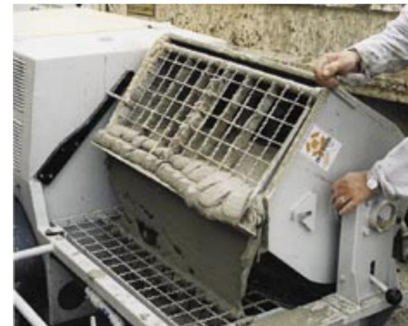
The swing mixer for the SP 11<sup>DMB</sup> is comfortable to operate and makes light work of difficult jobs.
