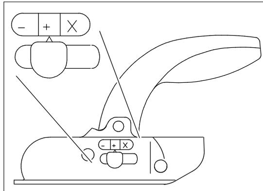
After correct engagement of the ball hitch, the pointer jumps to the green area of the marking, which is identified by a “+” sign.
