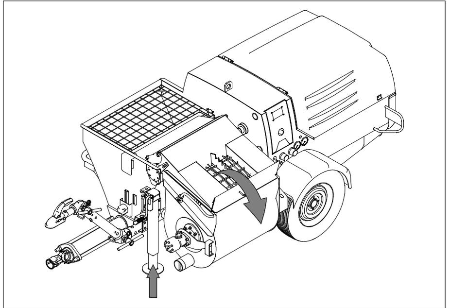
Lifting mixer unit in transport position
