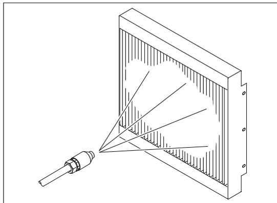
Spray the radiator down with a water jet
