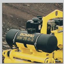
Two large-size corrosion-free water tanks for use on asphalt.
