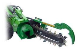
With trencher you can easily dig narrow trenches without damaging lawns and gardens – this trencher is ideal for smaller cable or pipe laying. Digging depth is max. 900 mm, digging width normally 100 mm or 150 mm, depending on chain type. Planetary drive with hydraulic motor guarantee efficient and trouble free operation. Three different types of chains available: standard earth chain, frost chain and heavy duty chain with tungsten teeth.
