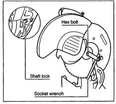
To install the blade, mount the inner flange, saw blade, outer flange and hex bolt onto the spindle in that order. Tighten the hex bolt by turning clockwise while pressing the shaft lock. Return the safety cover and center cover to the original position. Then tighten the hex bolt clockwise to secure the center cover. Lower the handle to make sure that the safety cover moves properly.
