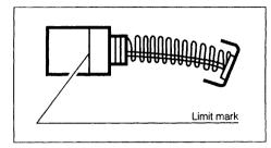
Use a screwdriver to remove the brush holder caps. Take out the worn carbon brushes, insert the new ones and secure the brush holder caps.
