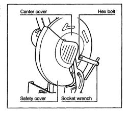
Press the shaft lock to lock the spindle and use the socket wrench to loosen the hex bolt by turning counterclockwise. Then remove the hex bolt, outer flange and blade.
