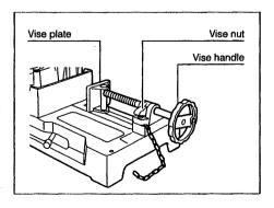
Long workpieces must be supported by blocks of non-flammable material on either side so that it will be level with the base top.
